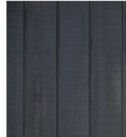
Thermally modified timber boards and structural sections to be used for the bird hide and lake tower cladding
